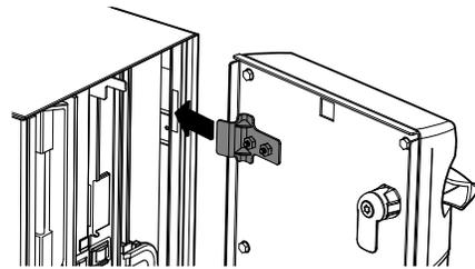
Hold door so that tabs are aligned with slots in cabinet.
